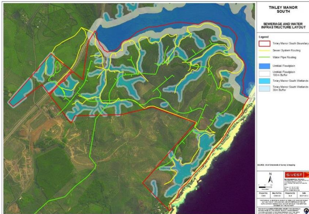
Figure 14: Sewerage and water infrastructure routing and wetlands.
