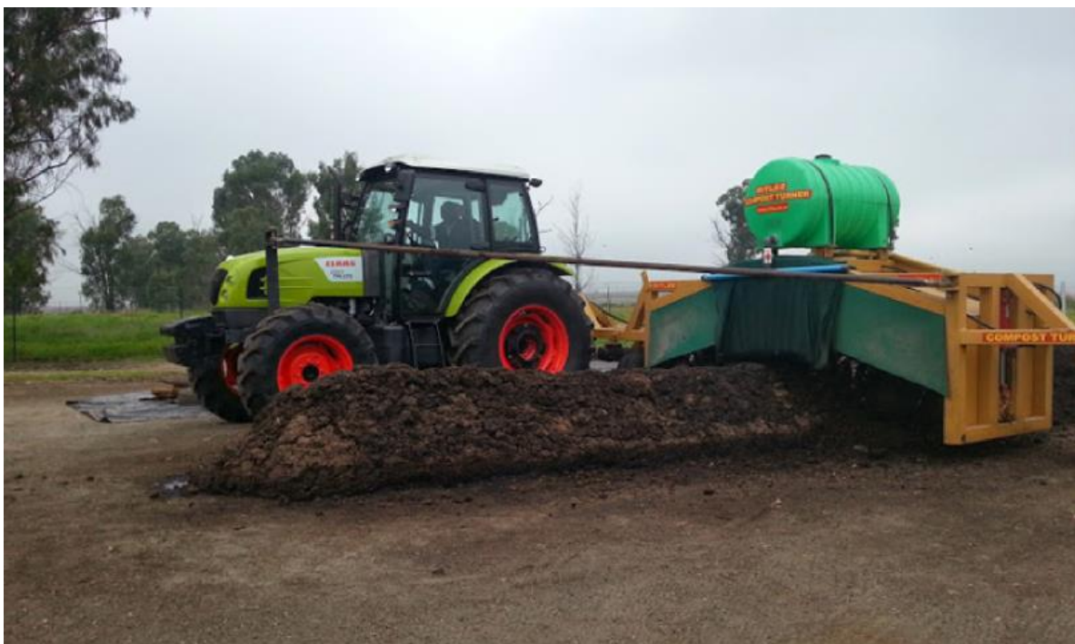
Figure 8: Windrow turning in order to aerate the compost
