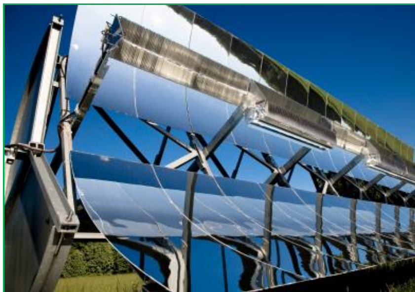
Figure 1-2: Example of a parabolic trough system.
