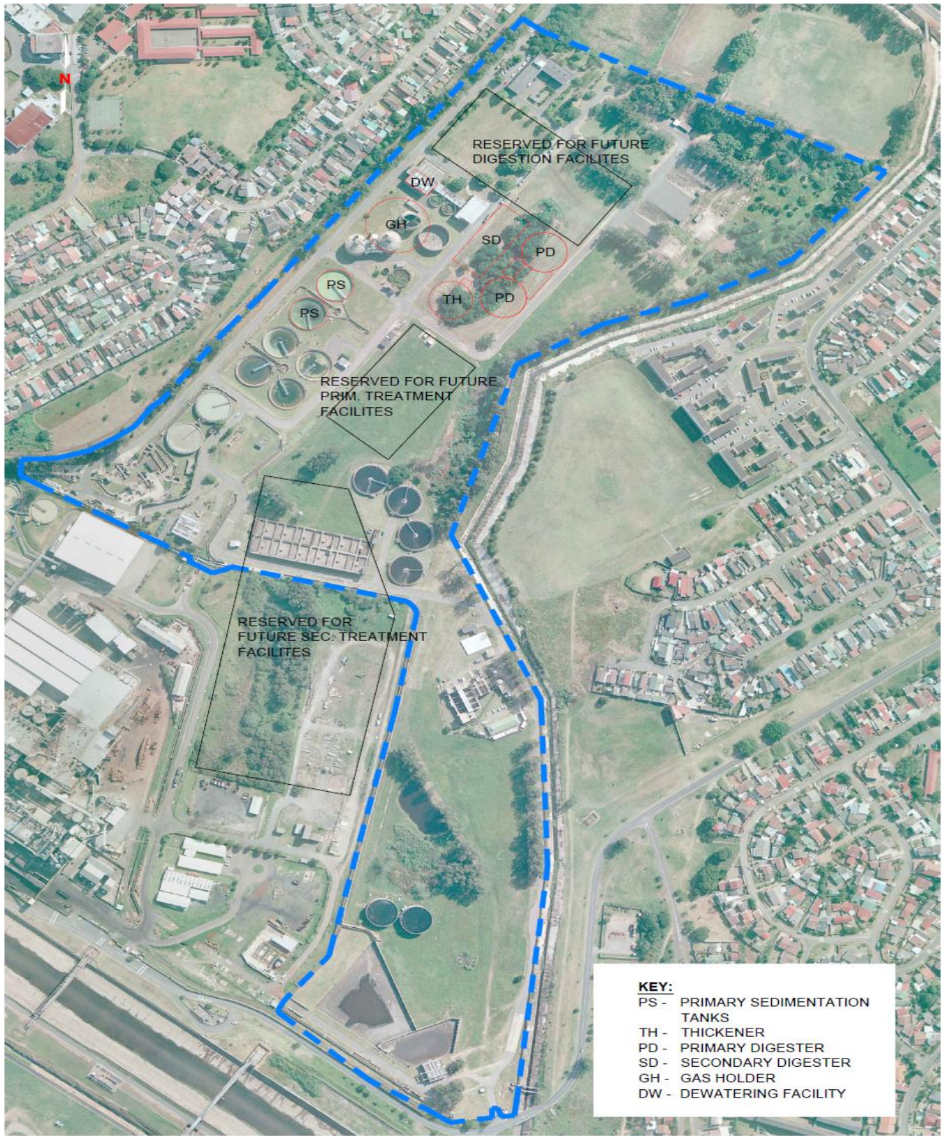
Figure 5-2: alternative 2, demolition of old sludge handling facilities and construction of new facilities
