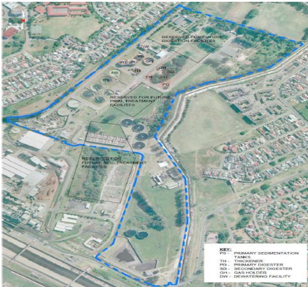
FIGURE 1: SWWTW AND LAYOUT OF PROPOSED UPGRADE FACILITIES
