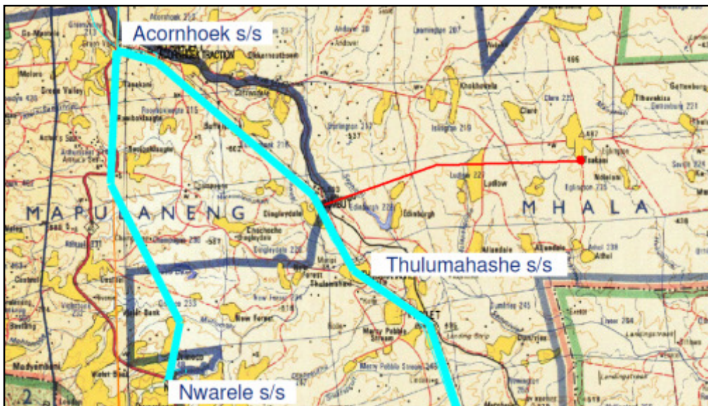
Figure 2: Zoomed in map of the Green Valley Network area (red line indicating the proposed power line connecting Mbumbu to Tsakani Substation)
