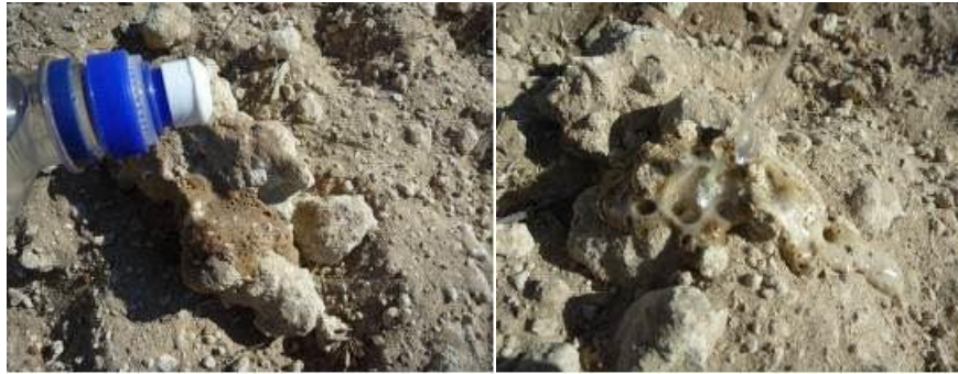
Figure 65: Addition of HCl (10 % solution) to subsoil lime and effervescence confirming the presence of carbonates
