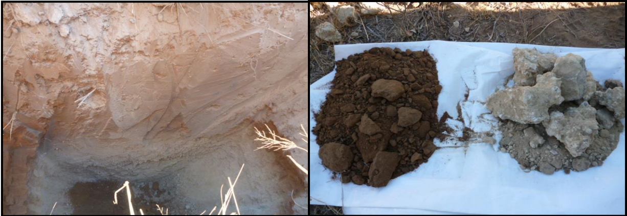
Figure 17: Aeolian sandy soils underlain by calcrete (left) and colluvial soils and nodular calcrete (right)
