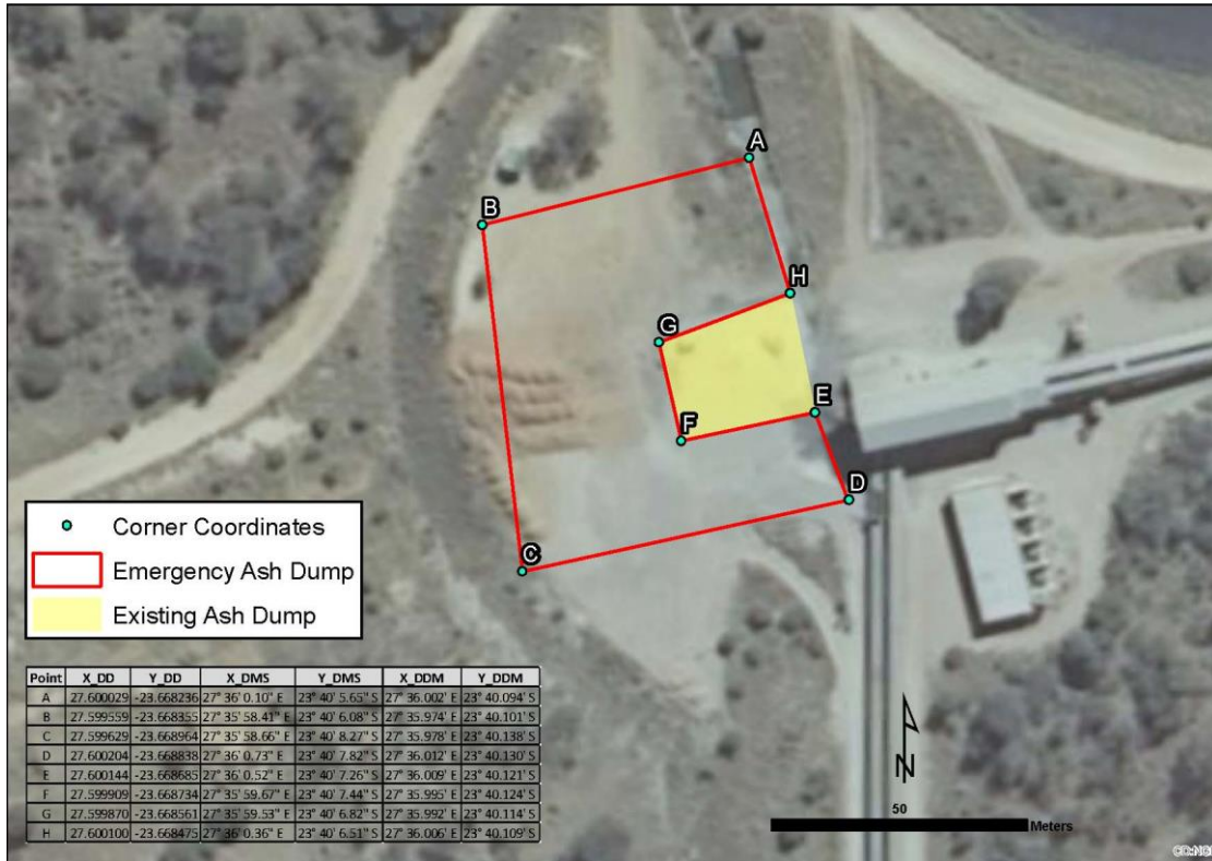
Figure 5: Google Earth™ image of the proposed expansion of the emergency ash offloading area and coordinates
