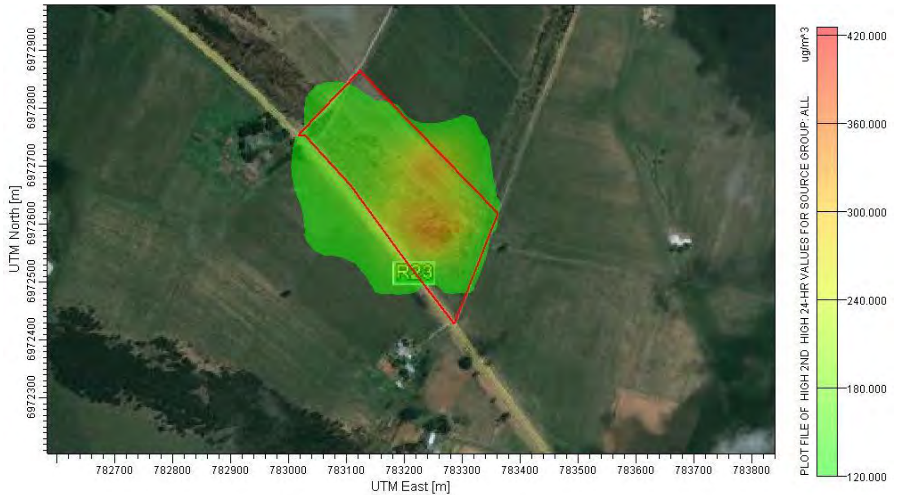
FIGURE 21: PREDICTED IMPACTS ASSOCIATED WITH DIESEL PARTICULATES FOR A 24 HOUR AVERAGING PERIOD (STANDARD 120 \mu\text{G}/\text{M}^3 ).
