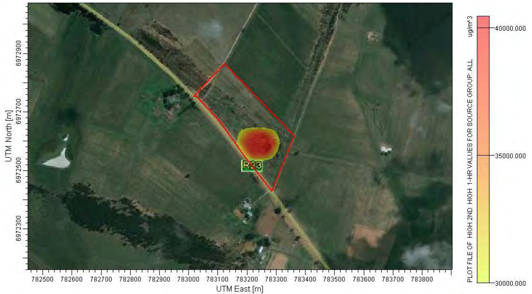
FIGURE 18: PREDICTED IMPACTS ASSOCIATED WITH CARBON MONOXIDE FOR A 1 HOUR AVERAGING PERIOD (STANDARD 30 000 \mu\text{G}/\text{M}^3 ).
