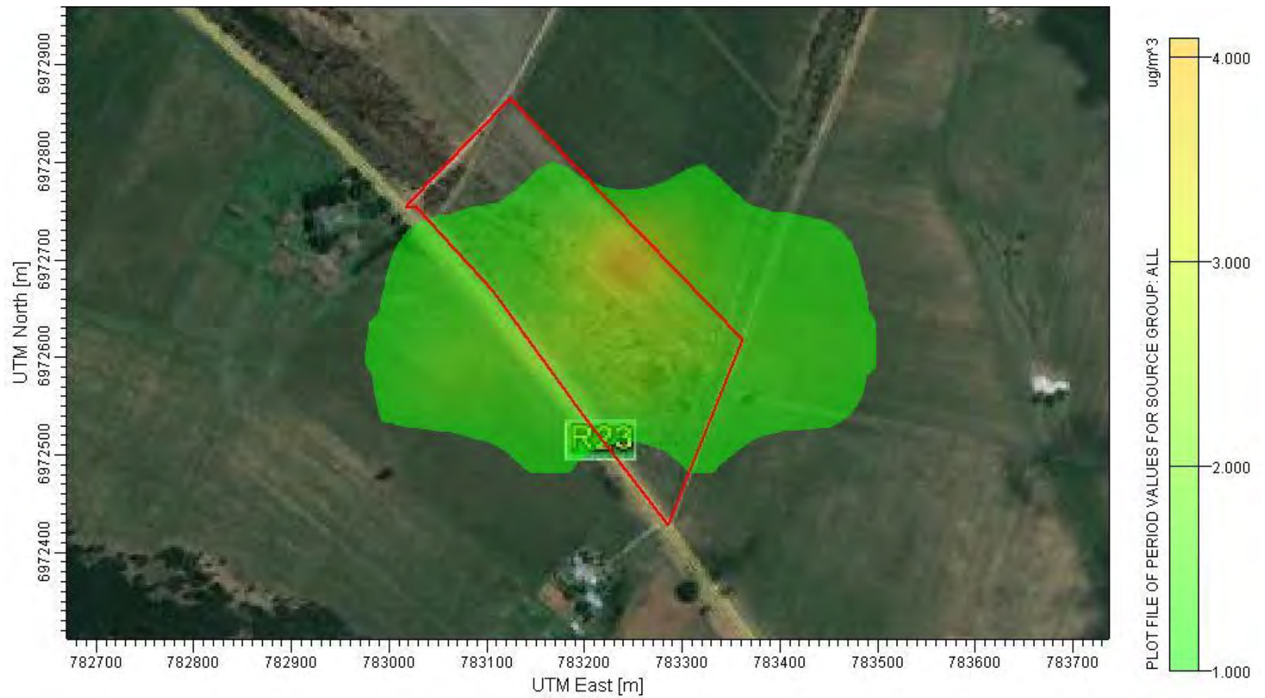
FIGURE 17: PREDICTED IMPACTS ASSOCIATED WITH BENZENE FOR AN ANNUAL AVERAGING PERIOD (STANDARD 10 \mu G/M 3 )
