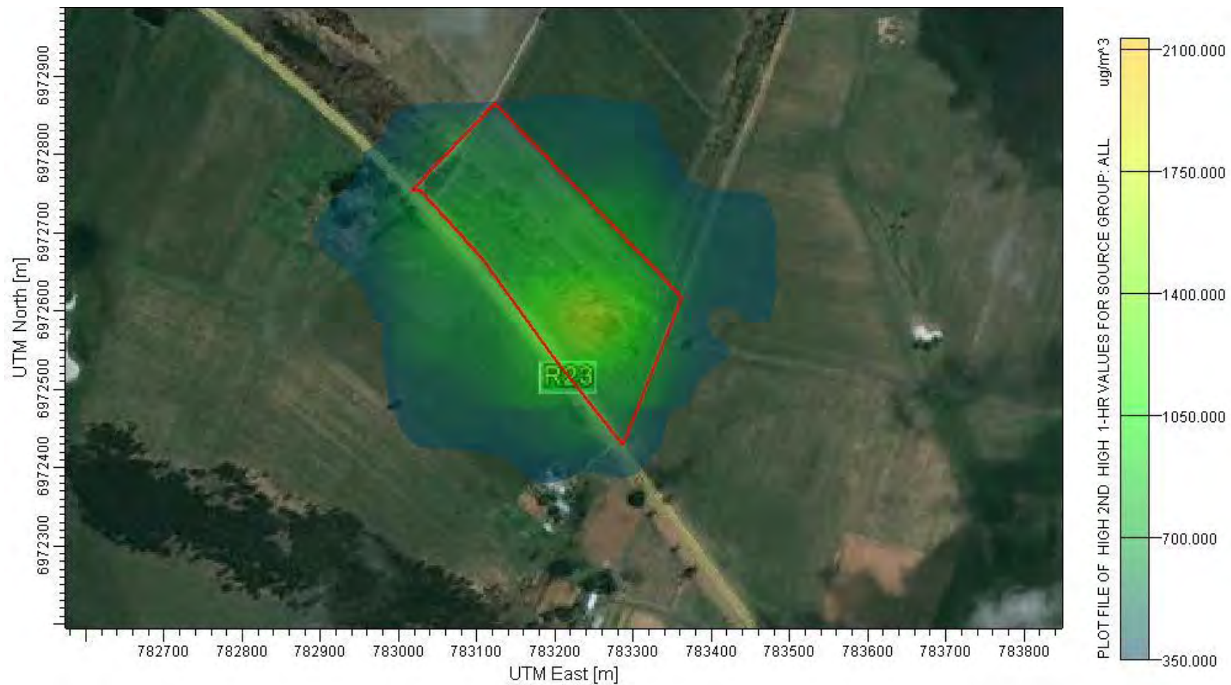
FIGURE 23: PREDICTED IMPACTS ASSOCIATED WITH SULPHUR DIOXIDE FOR A 1 HOUR AVERAGING PERIOD (STANDARD 350 µG/M³).
