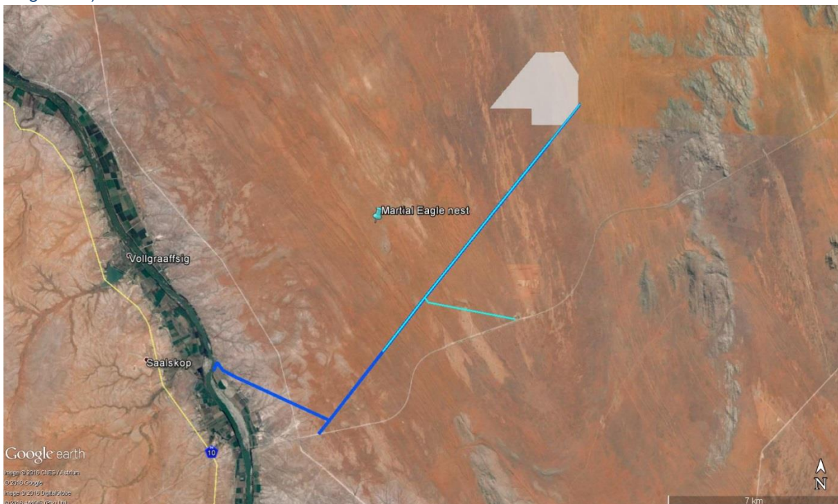
Figure 46: Recommended layout to minimise disturbance impact on pair of Martial Eagles breeding on tower 22 of the Garona-Gordonia 132kV power line
