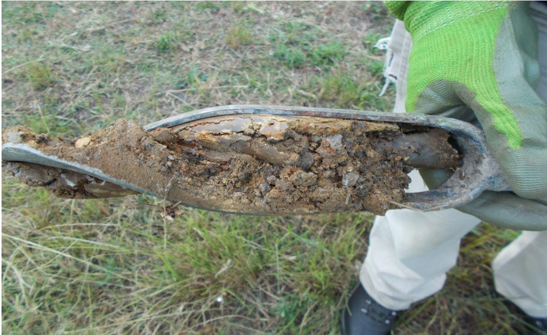
Figure 5 – Soft plinthic soils from a sample point
