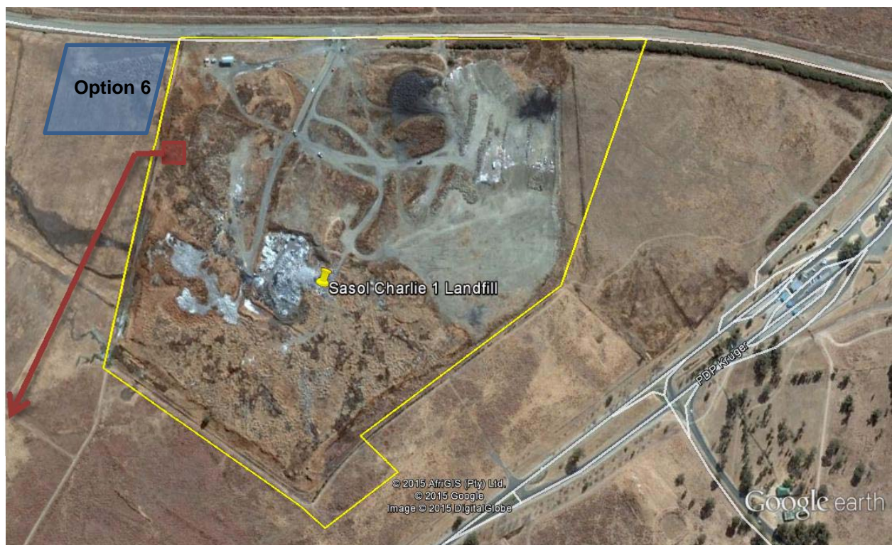
Figure 7: Option 6 involves pumping leachate to sewage treatment plant while stormwater run-off is collected in a new dam
