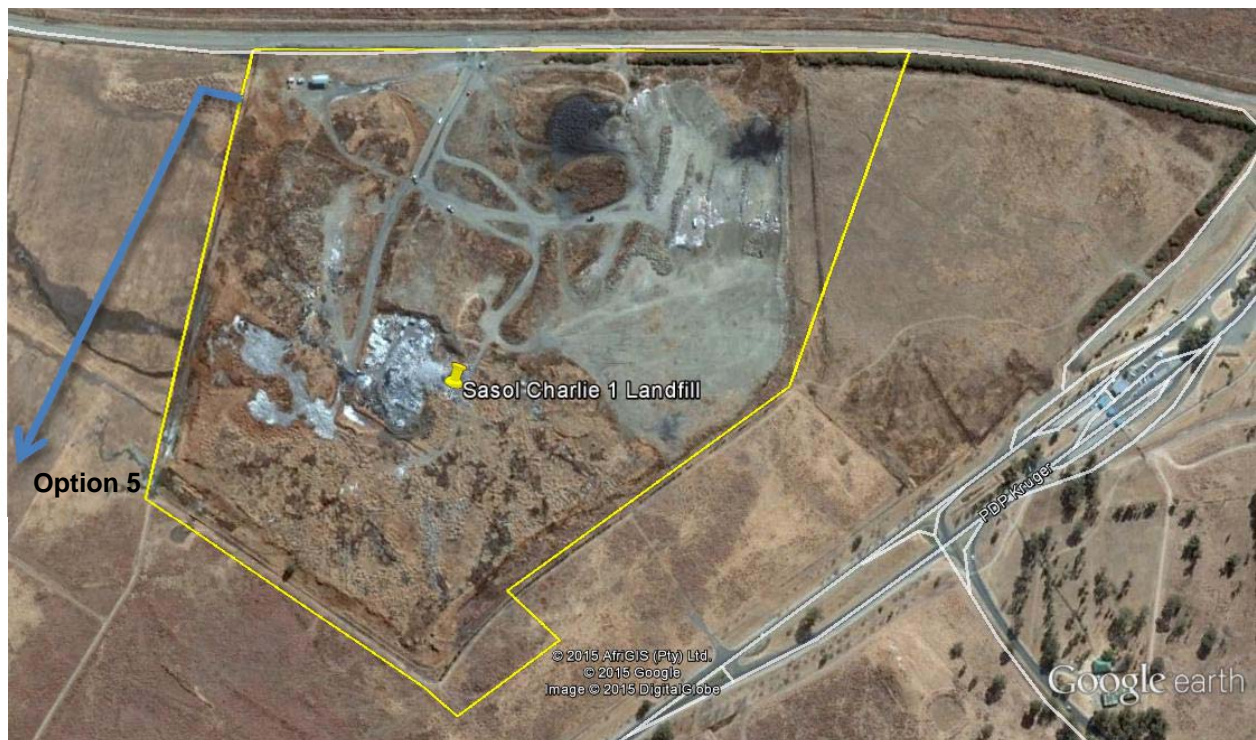
Figure 6: Option 5 involves pumping surface water and leachate to the sewage treatment plant
