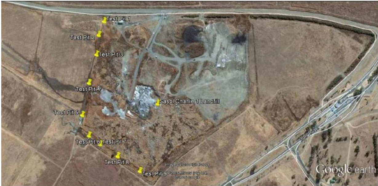
Figure 7: Test pit locations
